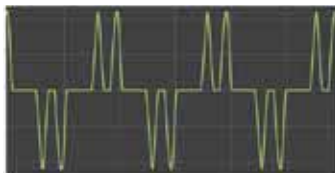
Motor drive without DC choke THDi 107%
