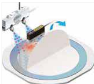
Measuring surface potential when removing BG sheets
